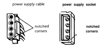
The power supply socket is on the back of the hard disk drive, next to the cable you just connected. The socket also has two notched corners, as shown above.
